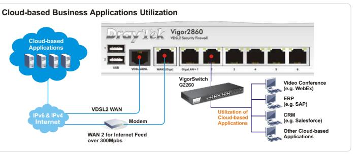
With two built-in modems, you have the flexibility of migrating to VDSL2 when your ISP/Telco upgrades from current ADSL2+ technology. Besides, in case you move to a new location where VDSL2 is not available, your router can fall
