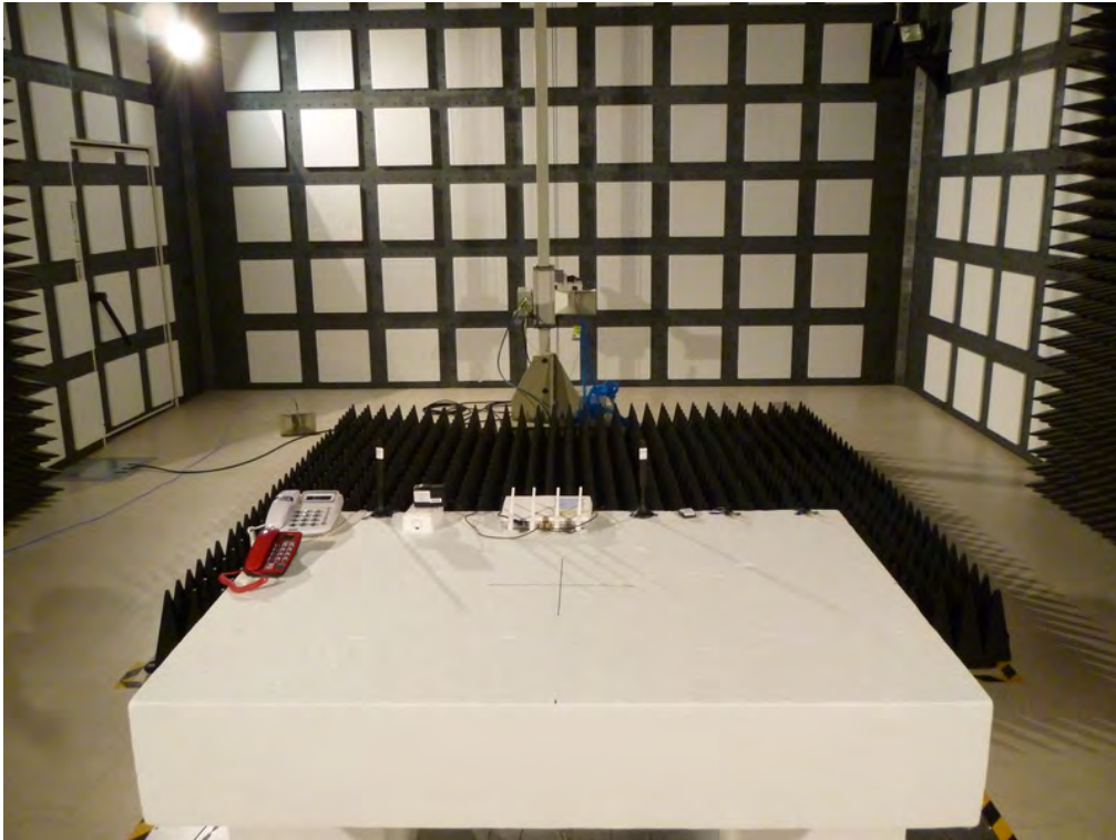
Radiated Emission - Rear View Above 1GHz (Mode 11)
