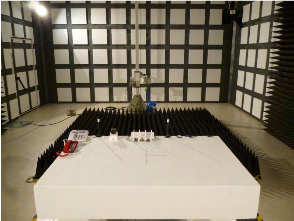
Radiated Emission - Rear View Above 1GHz (Mode 12)
